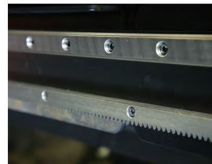
Helical Gear Rack with AGMA 12 grade ground pinions.
