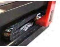
**Tuck Rail Design** Protects linear bearings, cable carrier, cables and hoses from harsh environments.
