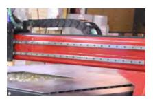
Heavy-duty Linear Bearings both "X" & "Y" Axis Provide smooth and accurate motion
