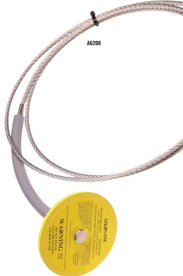
The 5K Drop Through Anchors – 8.5' overhead anchorage connectors have a 5,000 lbs. capacity. They are designed to drop through a 2" opening in an appropriate concrete or steel substrate. They are compliant with all ANSI® Z359.1-2007 regulations, and are available in custom lengths upon request.
