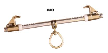
Light, smoothe and easy to use, Adjustable Beam Walkers are designed for fall protection, rope access, and work positioning. All models are constructed with lightweight aircraft aluminum bars and 360° swivel D-Ring connectors. The clamps attach without tools to I-Beams either overhead or underfoot. All models have a minimum breaking strength of 5,000 lbs.
