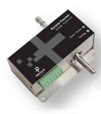
The Particles Plus® 2510-1 Remote Particle Counter measures 0.5  $\mu$ m and 5.0  $\mu$ m with a flow rate of 1.0 CFM (28.3 LPM). Integration is easy into a real-time monitoring or building management system via Modbus RTU. The 2510 models are the smallest 1.0 CFM remote particle counters on the market and have easy mounting options. The Particles Plus® 2510-1 units comply with ISO 21501-4 and include a 1 year limited warranty.
