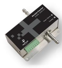
The Particles Plus<sup>®</sup> 2301-1 Remote Particle Counter measures 0.3 µm and 0.5 µm with a flow rate of 0.1 CFM (2.83 LPM). Integration is easy into a real-time monitoring or building management system via Modbus RTU. The 2301 models are the smallest remote particle counters on the market and have easy mounting options. The Particles Plus<sup>®</sup> 2301 units comply with ISO 21501-4 and include a 1 year limited warranty.
