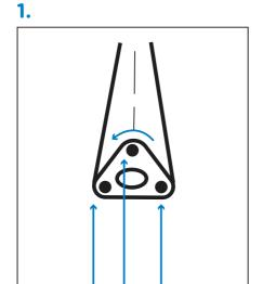
Unscrew 3 bolts on bottom side of centre column
