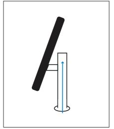
Adjust angle of display by loosening collar on top of bracket
