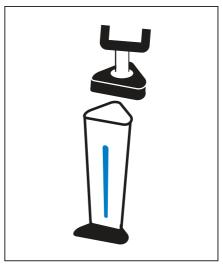
Fit monitor assembly to top of centre column and fix with 4 screws removed in step 2. Ensure display and centre column LED strip are aligned correctly
