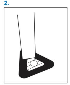
Insert centre column into opening on base plate being careful not to pinch cables
