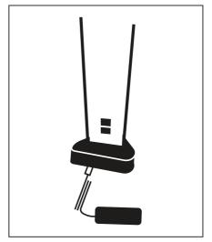
Insert 12v power lead to centre column to power on
