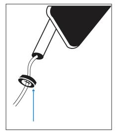
Remove lockring from display mounting bracket
