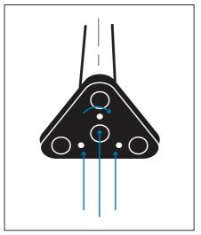
Insert 3 fixing bolts through baseplate to attach centre column
