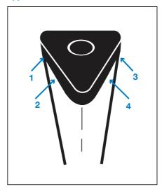
Remove 4 screws from top of centre column cap
